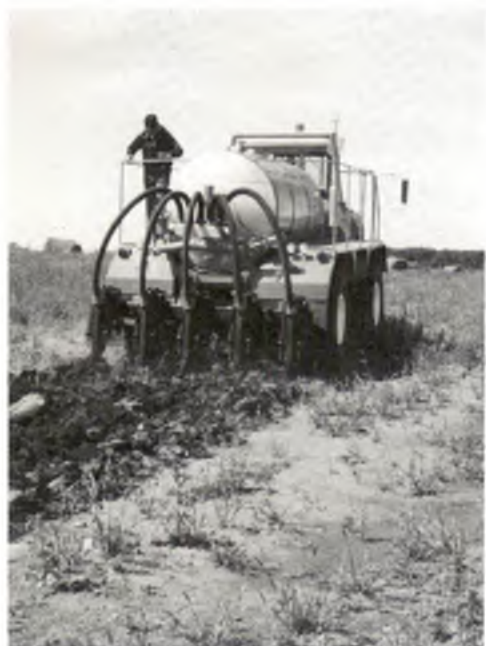
Harold Borstad, former utilities employee, standing on the back of the new sludge truck. Sludge is injected through lines at back of truck. Sludge from the plant goes to area farmers whose land meets EPA requirements for sludge application. It is distributed within a 5- to 13-mile area of the plant.
