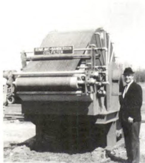
James Dornbush standing near a sludge vacuum filter installed in the late '60s as part of the renovation of the wastewater plant. Dornbush, an SDSU professor, maintained a close relationship with the wastewater department, providing advice and expertise through the years.
