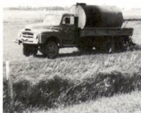
Sludge truck used in the 1970s. From the first, digested sludge was given to area farmers whose soil was suitable.
