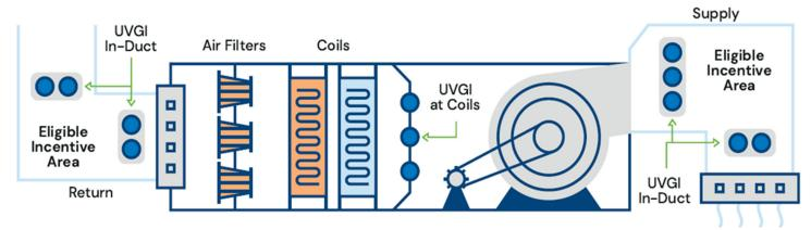
Note: UVGI at coils may be permitted if specifically designed for air pathogen inactivation.
